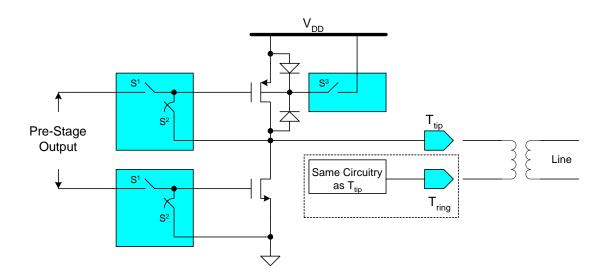
Figure 1 Simplified Block Diagram of the Transmitter Output Drivers
