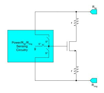
Figure 2 Simplified Block Diagram of the Receiver Inputs
