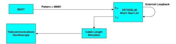
Figure 3 Simplified Lab Setup for Pulse Template Measurements
