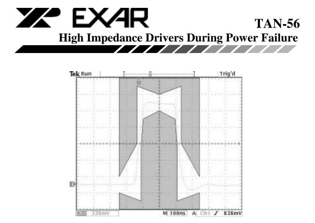
Figure 5 Pulse Template for E1 75ohm Impedance
